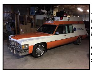
1977 Cadillac Superior Ambulance: #1 of 10 built in 1977. Overall Length is 244.55", 425 cubic inch engine. Was originally a demo unit for Wolfington Body Company, (Superior of Central NJ). Was in service with the Cheesequake Vol. First Aid Squad until April of 1994. In very good condition. Mike and Vicky were married during the 2004 PCS National Meet in Daytona Beach FL, and drove on the beach as husband and wife. The car won Best of Show at the event. Serious Offers considered.
